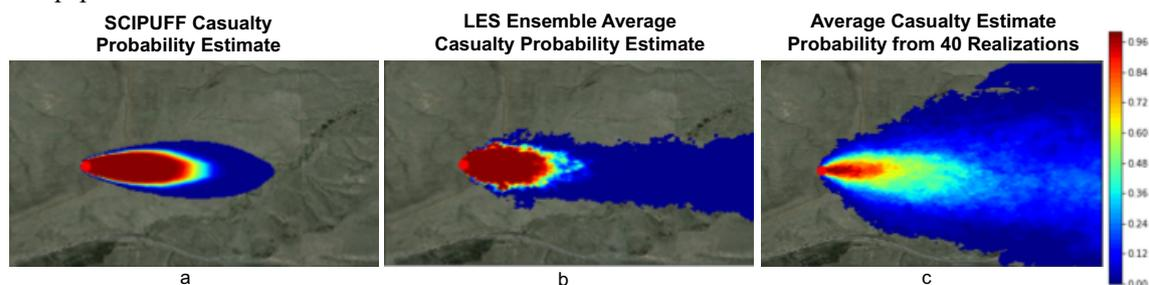
Figure 2. Two-dimensional casualty probability for a chlorine release in an unstable boundary layer. Figure a. is the estimate for SCIPUFF, figure b. is the estimate when averaging 40 realizations before the toxic load calculation, and figure c. is the casualty probability estimate from averaging the 40 realizations after the toxic load calculation.
