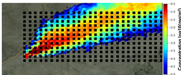
Figure 1. A GPU-LES dispersion solution for an urban stable PBL.
